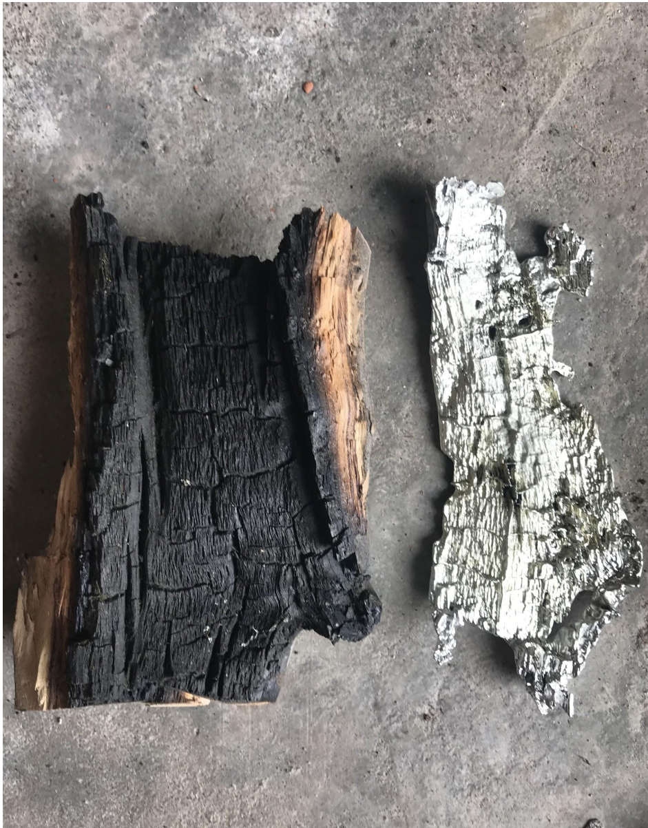
Olive tree that got burnt and the tin that got melted.
