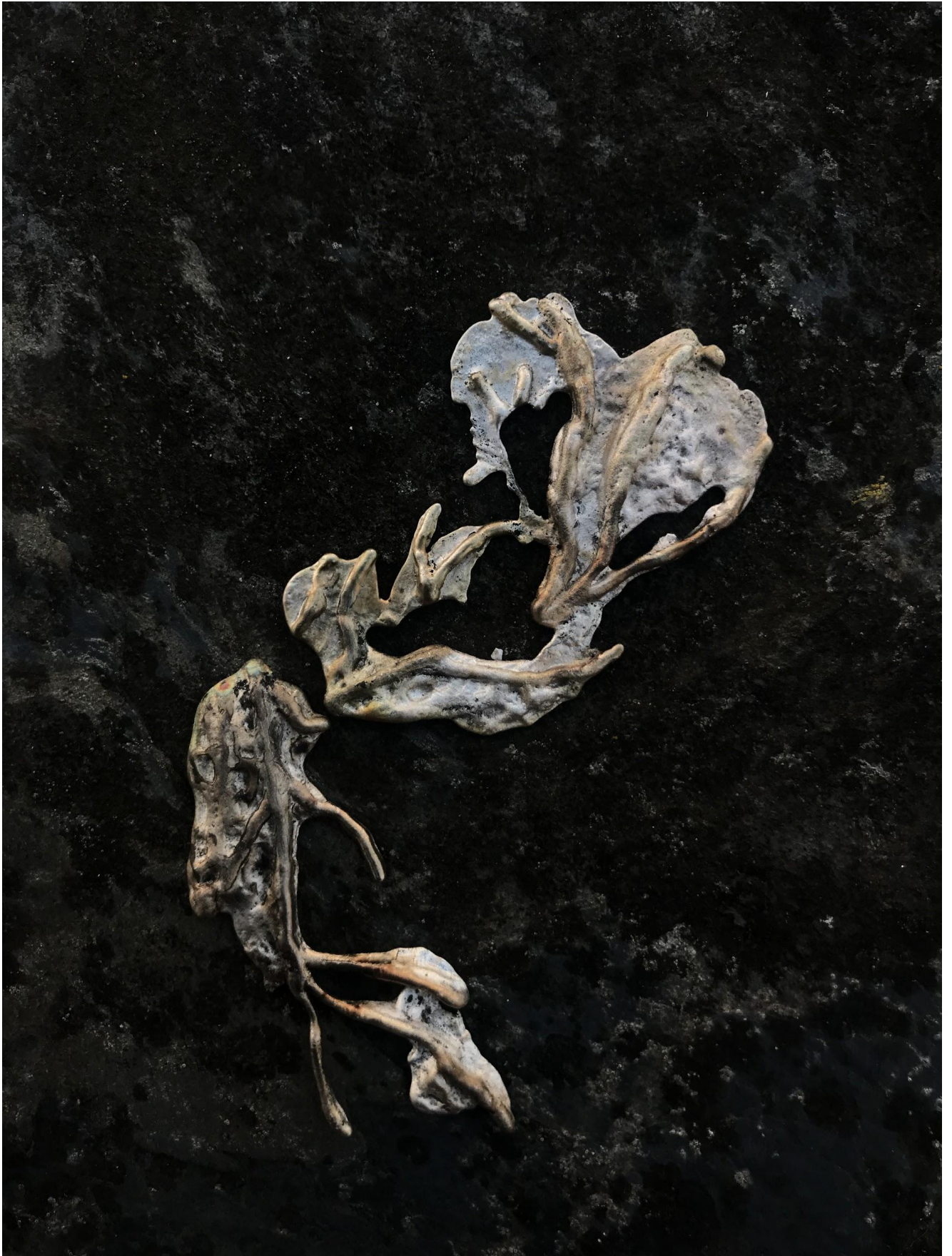
A cooled down silver that has flowed into the carvings. It hasn't flowed equally therefore looks broken.
