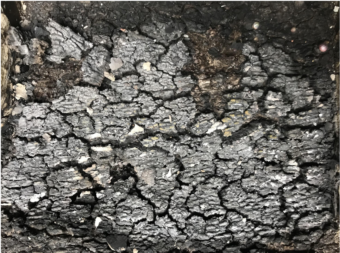
Cork bark is almost left to nothing after the casting of the bronze.
