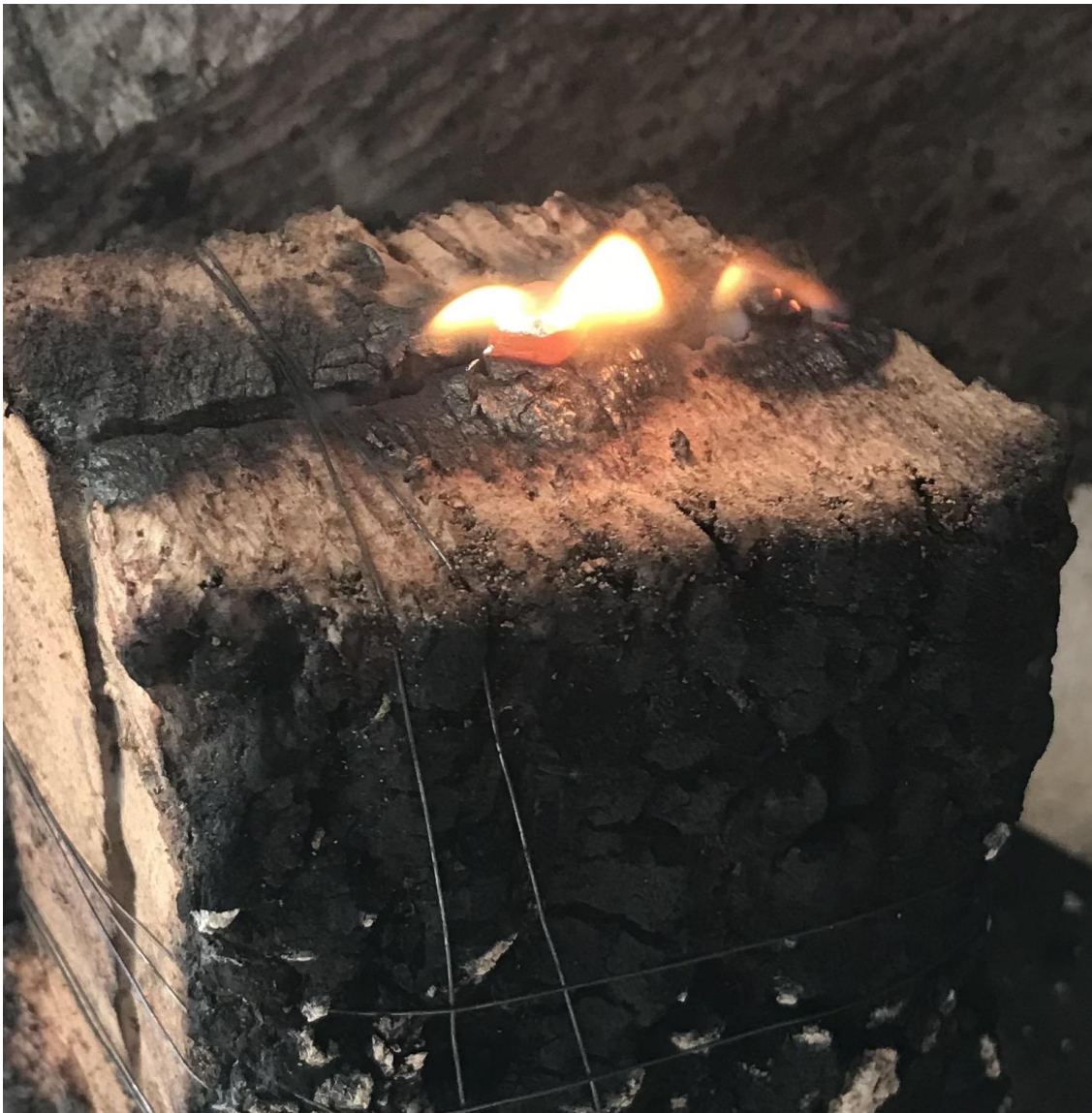
Hot silver in the cast form that is made of the first harvest of cork.
