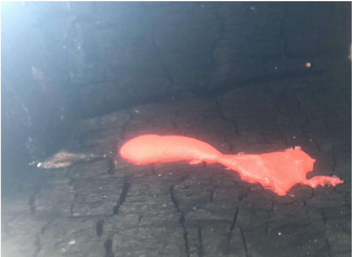
Freshly poured silver on the surface of the burnt wood, looking red.
