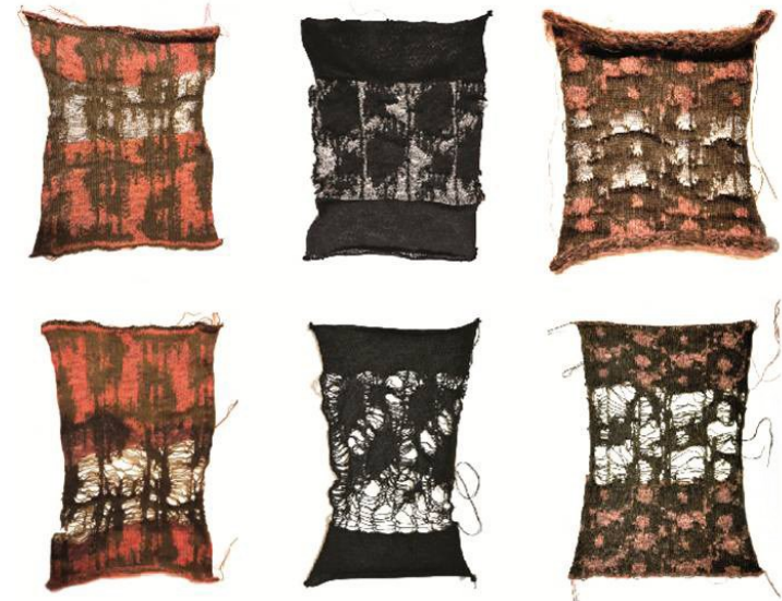
Above - Ravelling tests after the PVA has melted - Stoll ADF Below - Before and after the PVA has melted - Silver reed 840 Author's experiments
